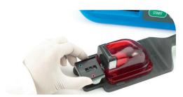
**Step 2:** Align the color-coded Tail Cover holes over the matching alignment posts of the Restraint Cartridge platform, and lower the Tail Cover over the tail allowing the magnets to securely seat it in place.
